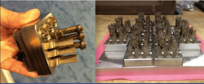
These direct metal laser-sintered parts, additively manufactured via an EOS M 290 system, have been “grown” onto small sub plates. This System 3R palletization concept allows parts created via AM to remain on sub plates through the balance of the machining process. Image courtesy Georg Fischer Machine Systems (GFMS).
